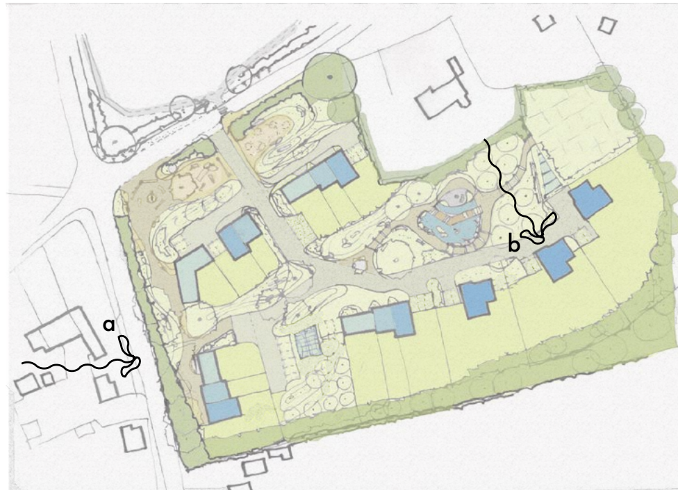
OPTION 1a: existing vehicular access off Common House Road retained and adjusted
